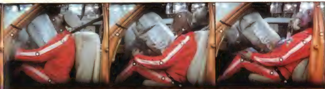
milliseconds it can sense a major frontal impact, inflate the driver's air bag, and tighten the front passenger's three-point seat belt.
